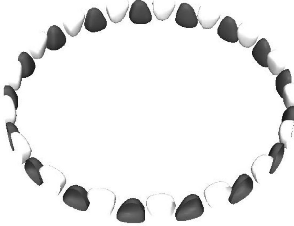
FIGURE 2. Isosurfaces of \Theta , at \Theta = \pm 0.05 , for m = 17 wall mode at Ra = 5 \times 10^4 , \Omega_0 = 625 and A = 0 . Movie 1, available in the online version, shows this solution over seven viscous times at a rate of 0.84 viscous times per second.
